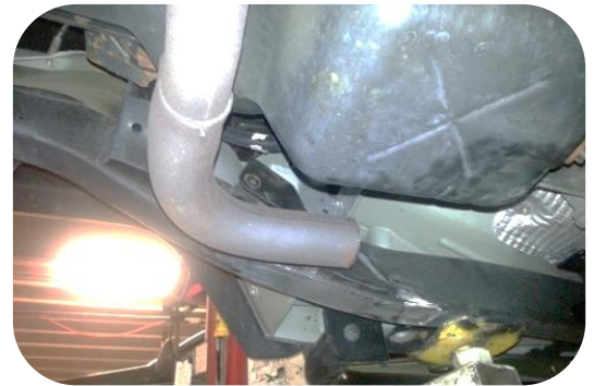
Figure 6 Exhaust after cutting.
