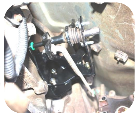
Figure 9 Transfer Case Linkage Installed
